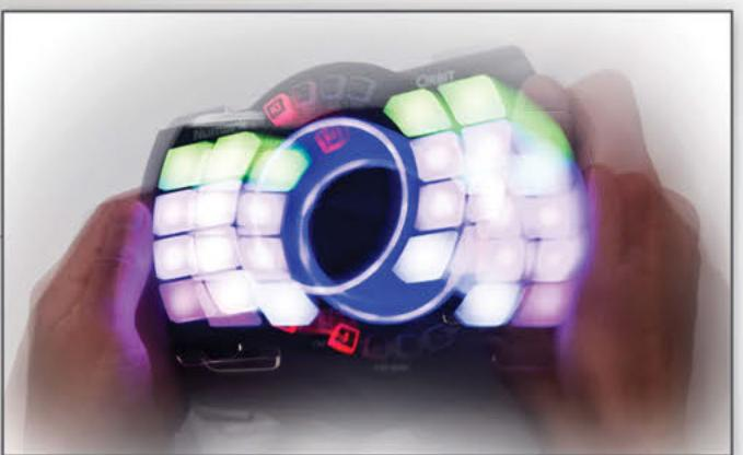
Built-in two-axis accelerometer allows manipulation of effects and filters by tilting forward, back, left, or right.
